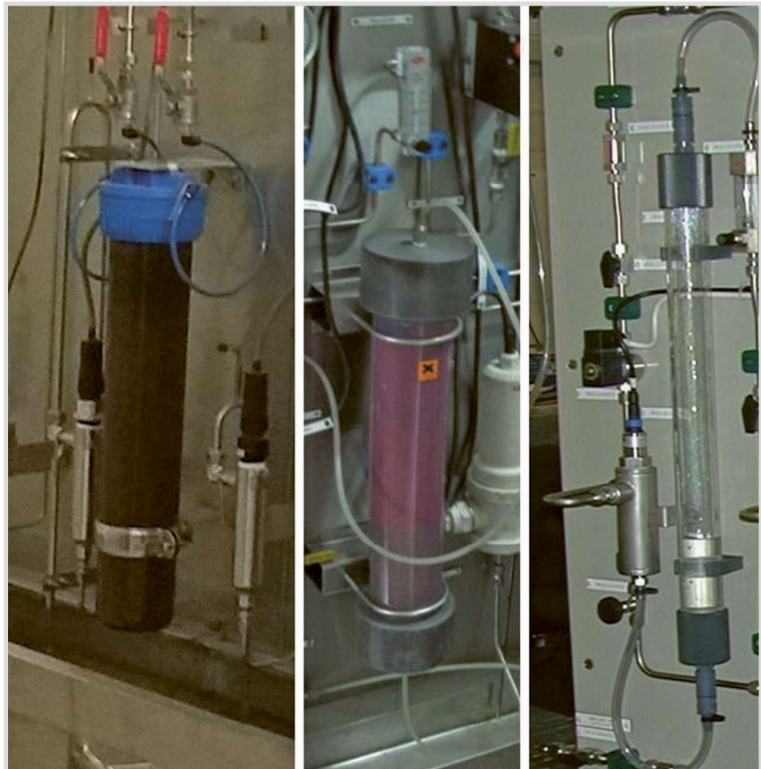
Fig. 3. Examples of variety of cation exchanger designs.
